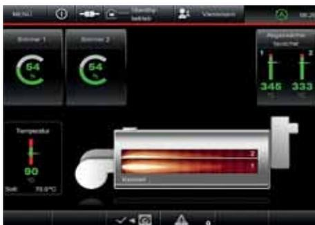
Vitocontrol HS being used with a Viessmann double flame tube boiler
