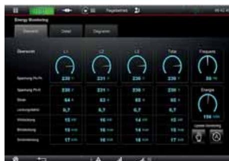
Energy monitoring shows the current boiler output at a glance.
