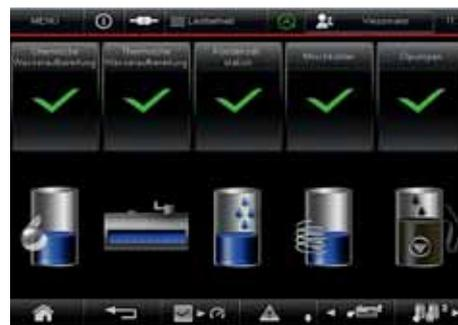
The Vitocontrol HS can also be used to control all auxiliary systems.
